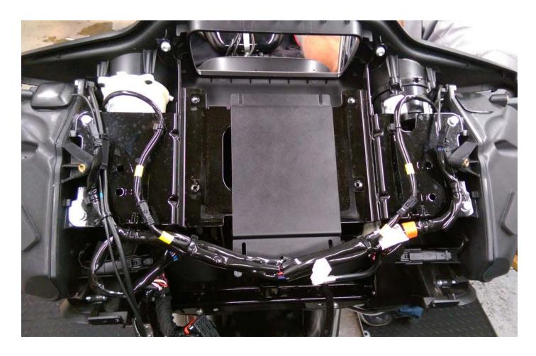
2. With the radio removed, you will see a large, black, steel bracket that is the main support for the fairing. The amplifier mounting place will lay on top of this support so that is it held in place by the radio when it is reinstalled.
