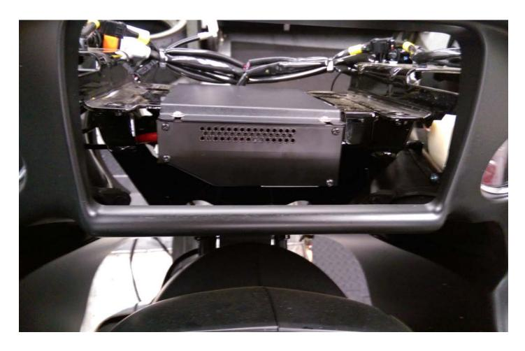
6. Looking through the opening for the radio, you can see the wiring exits on the left hand side (clutch level side). The steel structure around the amplifier is shaped perfectly to accept it with all the correct angles to provide clearance. Now would be a good time to insure the wiring is secure and will not abrade on anything metal.
