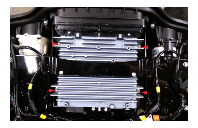
1. Rremove the stock radio. The amplifier will be located upside down beneath the radio.
