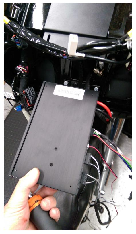
3. By now the amplifier should be completely wired and tuned. You will not be able to make any adjustments after this point without removing the amplifier. If needed temporarily reconnect the radio and test the system.
