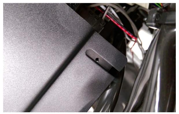
4 Secure the amplifier to the bracket using the provided screws and washers. Some Blue Locktite® would be a good idea here.
