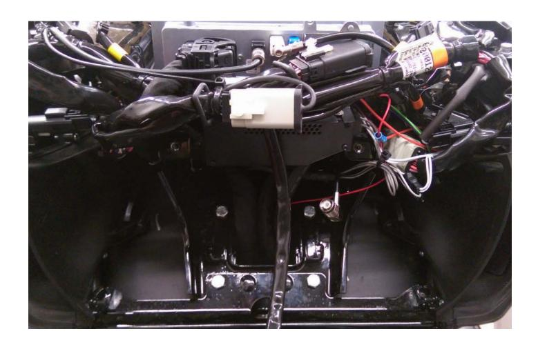
7. With the radio reinstalled and connected the finished amplifier installation should look like this. Make sure you have all the connections at the radio correct, fully seated and tightly secured. The system should now be ready for a final system check.
