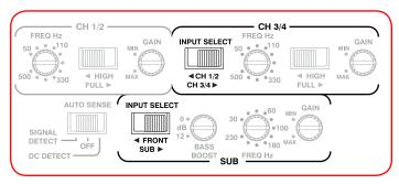
The SUB INPUT SELECT switch determines if the subwoofer channels are driven by the two SUB RCA inputs as when set to SUB mode, or from RCA Inputs 1 and 2 when in FRONT mode.
