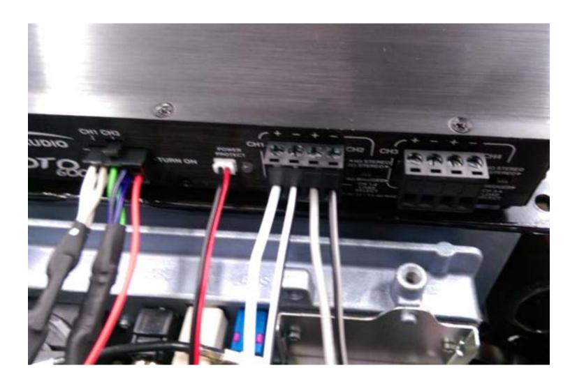
25. On the end of the speaker harness are 4 stripped wires. Connect them to the 4 screw block terminal on the end of the amplifier with the controls.
