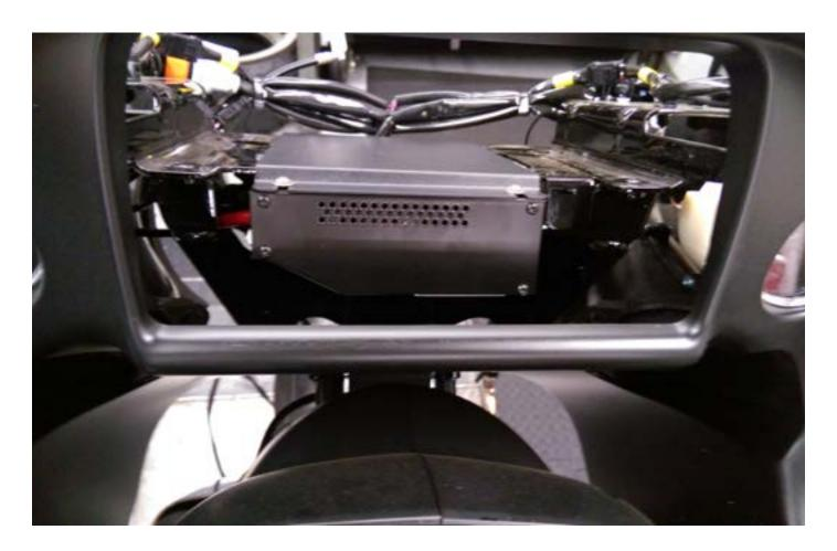
33. Looking through the opening for the radio, you can see the wiring exits on the left hand side (clutch level side). The steel structure around the amplifier is shaped perfectly to accept it with all the correct angles to provide clearance. Now would be a good time to insure the wiring is secure and will not abrade on anything metal.
