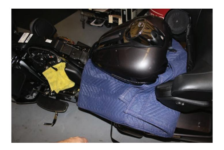
5. Short Cut. While it is advisable to remove the chrome "Dash Board" from the tank and fully disconnect all wires and lines attached, you can carefully swing the tank around and set it in the seat position. A great deal of care must be taken to insure nothing is scratched or damaged. If you are uncomfortable with this method, please watch the tank video below for complete tank removal instructions.
