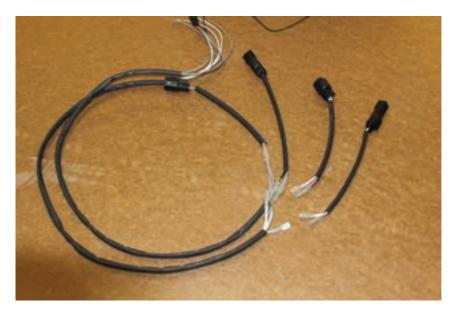
22. You now need to assemble the speaker harness. Just plug the adapters to the ends of the harness, matching the connectors with their appropriate mate. Make sure the insulating covers are firmly in place. A shorted wire here will shut down or possible damage the system.
