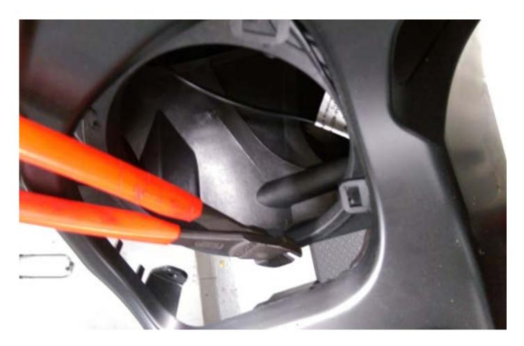
18. There is a plastic alignment pin, molded to the speaker housing. This must be trimmed flush with sharp flush cutters or a razor knife.
