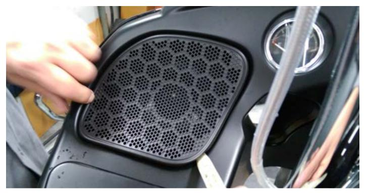
14. Remove the speaker grill by prying gently on the inner side. Then remove the 2 Torx head screws holding the fairing.
