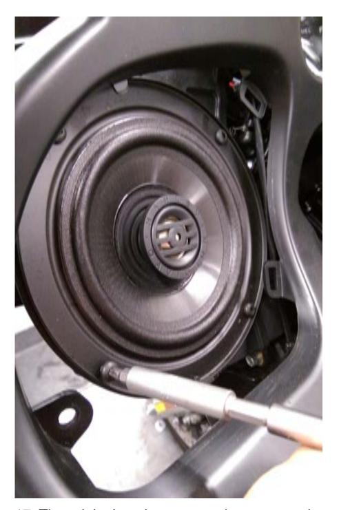
17. The original equipment speaker can now be removed and put aside. It will not be needed again. The 4 Trox head screws will be retained and used to hold the new speaker.
