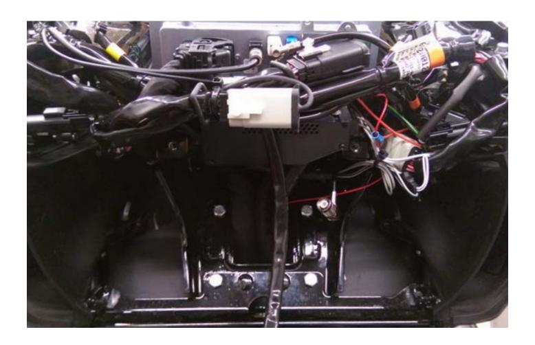
34. With the radio reinstalled and connected the finished amplifier installation should look like this. Make sure you have all the connections at the radio correct, fully seated and tightly secured. The system should now be ready for a final system check.
