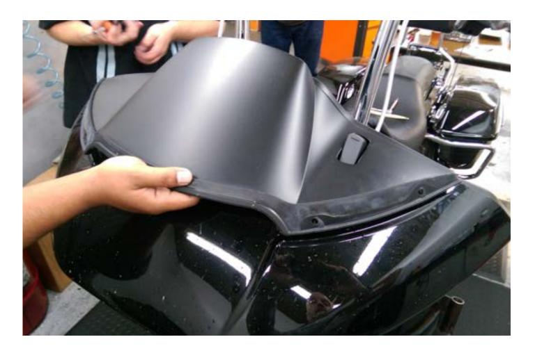
11. Remove the Upper vent assembly. No tools required here. It just pops off.
