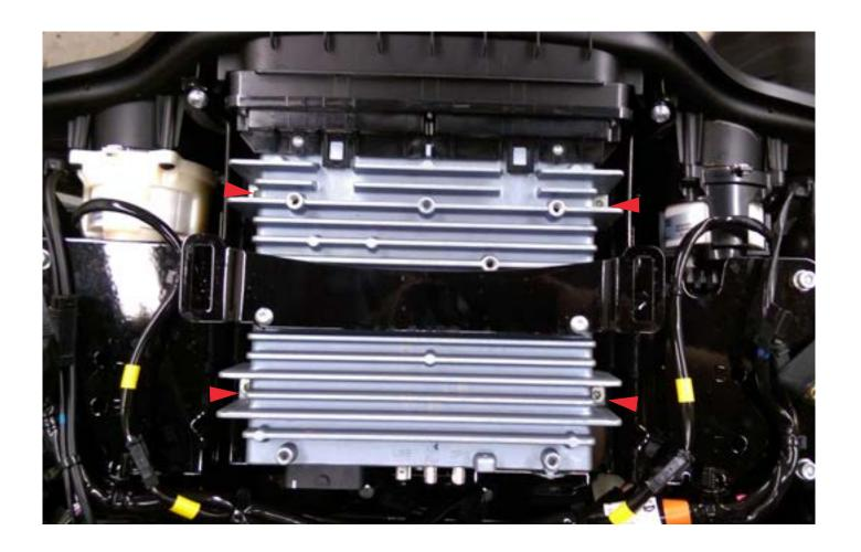
21. It's time to remove the stock radio. The amplifier will be located upside down beneath the radio.
