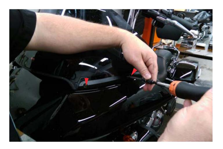
10. Remove the 4- Torx head screws below the windshield. Warning: The windshield will be loose and ready to remove. Don't let it fall.
