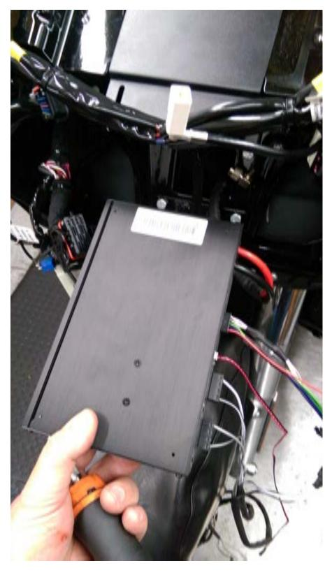
30. By now the amplifier should be completely wired and tuned. You will not be able to make any adjustments after this point without removing the amplifier. If needed temporarily reconnect the radio and test the system.
