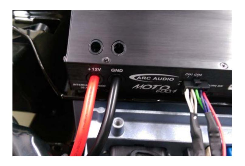
23. Connect the power harness from the battery to the 3 screw terminal block on the end of the amplifier. You did remember to remove the fuse from the harness right? The Red wire goes to the +12V terminal, black to GND and the
