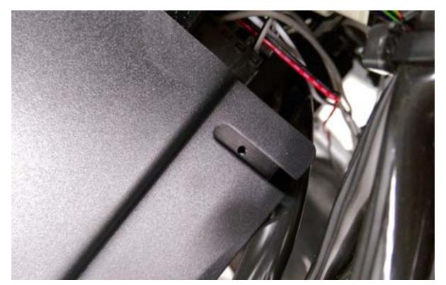
31 Secure the amplifier to the bracket using the provided screws and washers. Some Blue Locktite® would be a good idea here.
