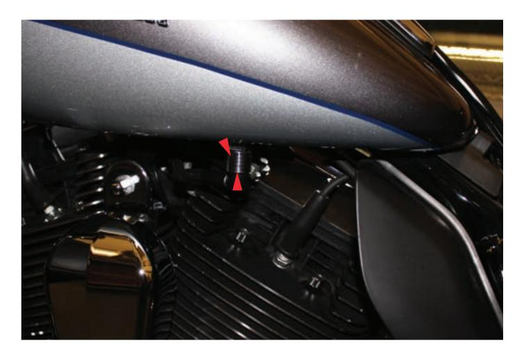
4. To disconnect the fuel line from the fuel tank, locate the quick disconnect fitting on the left side of the tank.
