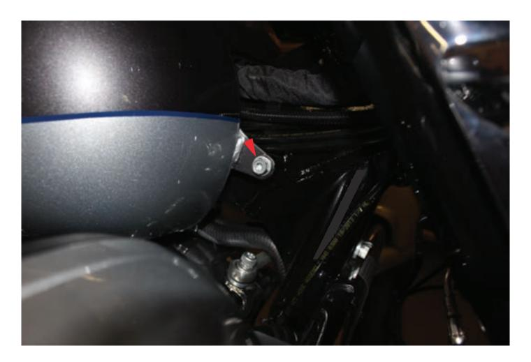
3. Remove the 2 bolts at the front of the tank. These are under rubber covers that must be removed first.
