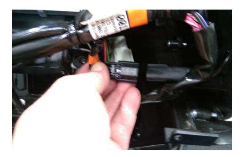
27. No tools are needed to make this connection. Make sure the connectors are fully seated and latched.
