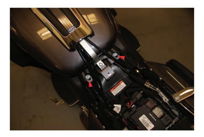
2. Remove the 2 bolts at the back of the tank under the seat. Don't drop them down by the battery. You will need them later.
