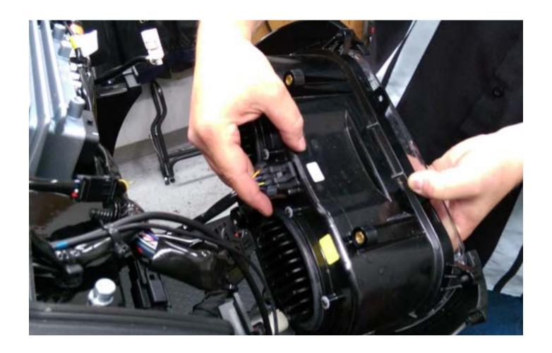
20. Remove the headlight by removing the 4 screws securing it to the fairing and unplug the harness. You will need access behind the headlight when mounting the amplifier.
