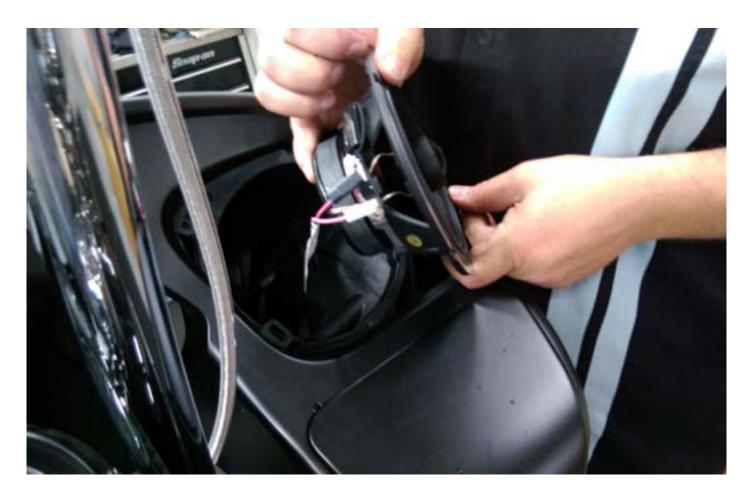
19. The new speaker can now be plugged in a installed. The Side connectors are sized to the correct plug, large and small. We have found some bikes require that the rubber magnet cover be removed from the speaker for clearance. This has no negative effect on the speaker and will not affect your warranty. Secure the speaker with the original Trox head hardware.
