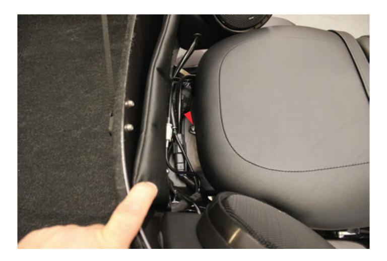
1. Locate the Philips head screw at the back of the seat and remove it being careful not to drop it. This will free the back of the seat. Raise it slightly and slide the seat toward the back of the bike until it comes free.
